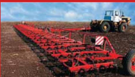
LIRA Hydraulic Spring-Tooth Wide Level Harrows
