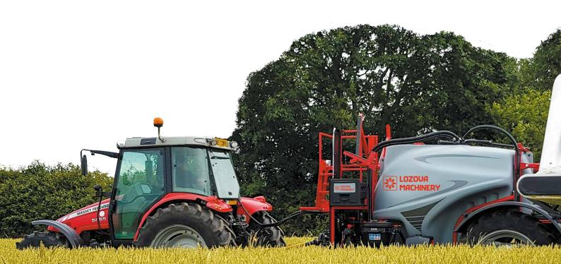
The high-lift parallelogram frame and the boom's suspension system results in a level ride boom for accuracy and performance
