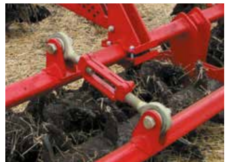
Roller adjustment for choosing the tillage type
