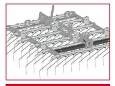
Central adjustment of the attack angle of the teeth
