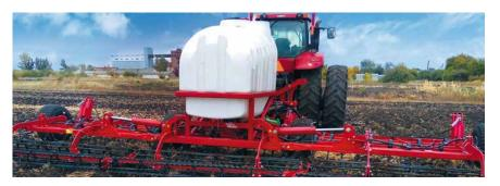
CHERVONETS XL with module for applying liquid fertilizers
