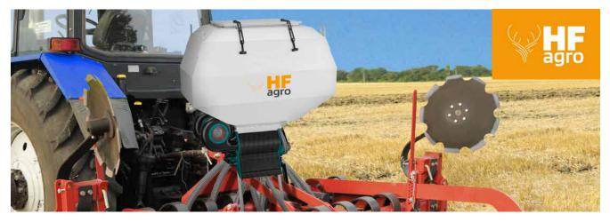
DUCAT disc harrow can be equipped with an additional module that allows you to apply granular fertilizers, as well as use it for overseeding (for example, green manure) in one pass with the main processing.
