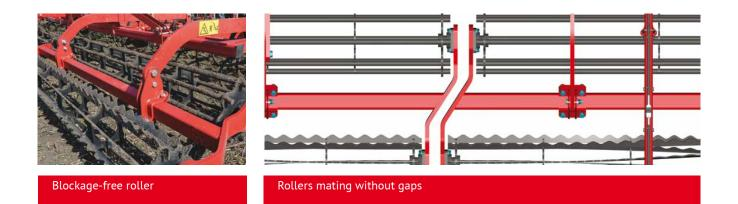
The roller has no central axle, thus there is no roller blockage even in overwatered conditions. Front and rear rollers have different diameters and rotation speeds, providing the finer soil fraction.
