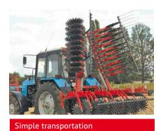
Hydraulically folded frame ensures the harrow compactness in transport position and minimizes loads on the tractor linkage. Transport width is 3 m.
