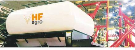
Module for applying granular fertilizers
