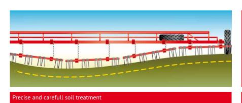
Having the chained individual working sections, the LIRA spring harrow perfectly follows any field contours in spite of its wide working width.
