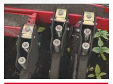
Two-stage adjustment of pressure
