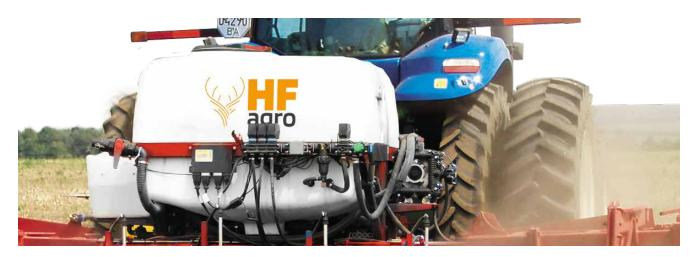
The SHILLING can be equipped with an additional HF Agro module for applying basic and starting liquid fertilizers simultaneously with the main operation of the unit.
